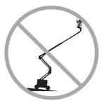
Do not raise or extend the boom unless the machine is on a firm, level surface. Do not depend on the tilt alarm as a level indicator. The tilt alarm sounds in the platform only when the machine is on a severe slope.
